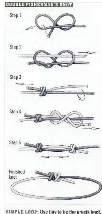
The knot on the left shows how to tie the ends of the line to make the SafeTree Prussik Loop. This is the most effective knot to keep it together.
