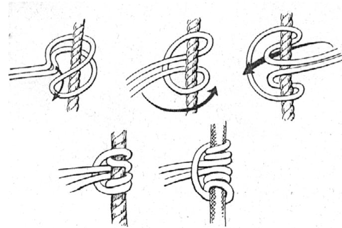
The above diagram shows how to tie the Prusik knot, which is used to connect the SafeTree Loop to the SafeTree Climber line.
